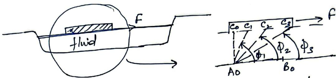
Continuous shear deformation under the action of constant shear.
