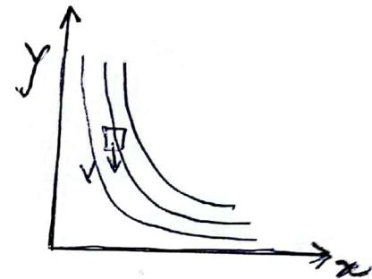
So, Given  $\vec{V} = \vec{V}(x, y, z, t)$  find the acen. of a fluid particle  $\vec{a}_P$
